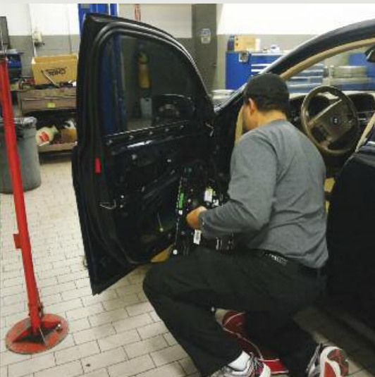
(Below from Left) Using an instructional video displayed on a tablet, John Walker replaced the driver's side window regulator on his 2005 745Li. (Middle) Chris Wootten kindly helped out a few club members by reading diagnostic information and unlocking special codes using the MyCarly app on his phone. (Right) The rotors on Michael Cammill's Z4 were rusted in place, but with the persuasion of a hammer, they were set free.
