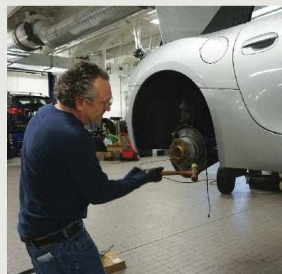
(Below from Left) Using an instructional video displayed on a tablet, John Walker replaced the driver's side window regulator on his 2005 745Li. (Middle) Chris Wootten kindly helped out a few club members by reading diagnostic information and unlocking special codes using the MyCarly app on his phone. (Right) The rotors on Michael Cammill's Z4 were rusted in place, but with the persuasion of a hammer, they were set free.
