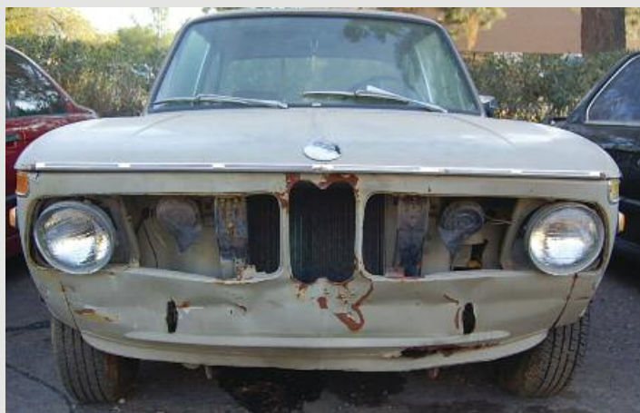
(Above) Since the car arrived with a severely damaged front end missing grilles and a bumper, new components were sourced (Right).
