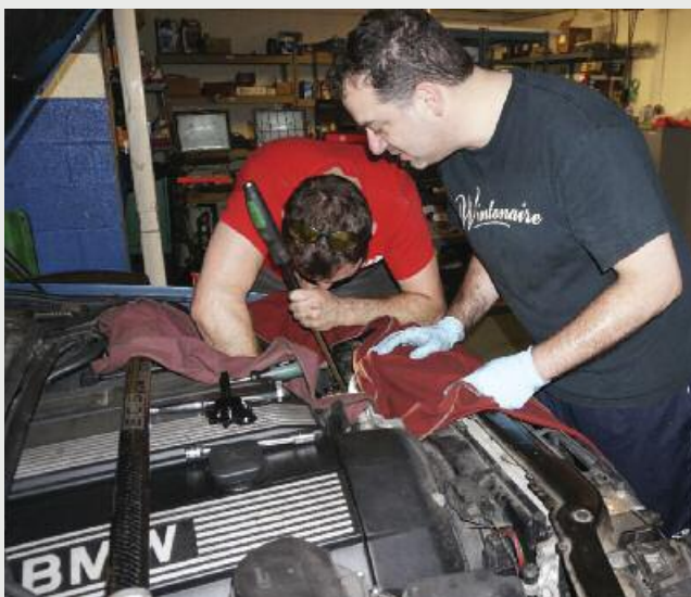
(Top) Frank Kapitan had to remove the rear bumper cover on his X3 in order to mount a new trailer hitch. (Above) Brian Lovecchio and Shop Foreman Andrew Goodnight work on replacing the power steering hoses on Brian's 330ci.
