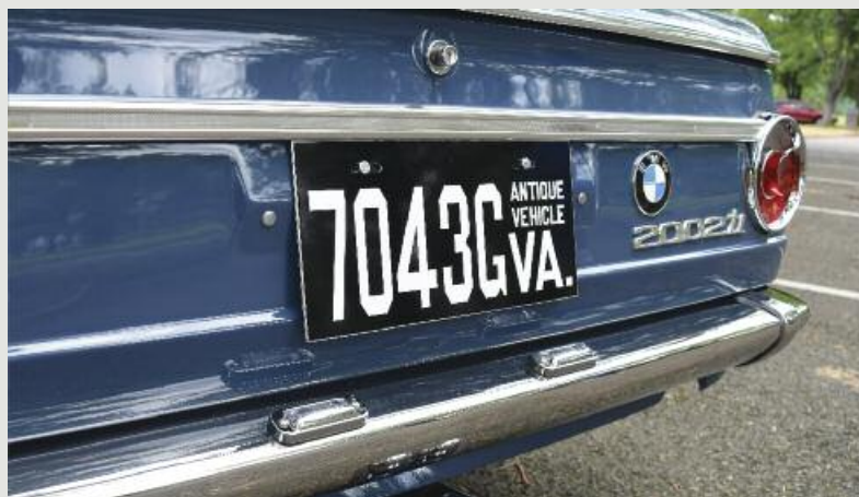
(Below) Rear shows removal of USA-specific reflectors and tag lights. New European-type bumper has integrated tag lights.
