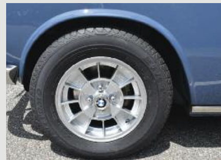
(Above) A set of Ronal 13" alloy wheels with 185 series radial tires replace the original stamped steel units for better looks and handling.
