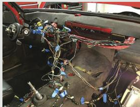
Wiring harness view 3 (helps in reassembling the dashboard)
