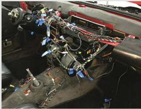
Wiring harness view 1 (this is important for reassembly)
