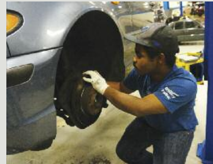
(Bottom left) The owner of this Porsche 944 racer towed it by trailer almost 12 hours so it could be analyzed and tuned on ASM Performance's Dynapak dynameter. Note how the rear wheels have been removed and the machine attaches directly to the hubs rather than the wheels spinning on rollers. (Bottom right) Tyrik Dedrick helped his Mom out by replacing the front brake pads and rotors on her E46 3 Series. (Middle right) John Walker replaced the side running boards on his X5.
