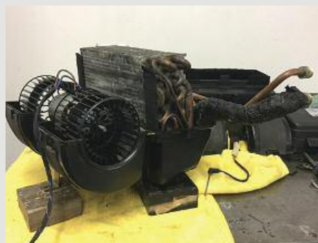
Evaporator with circulating fans
