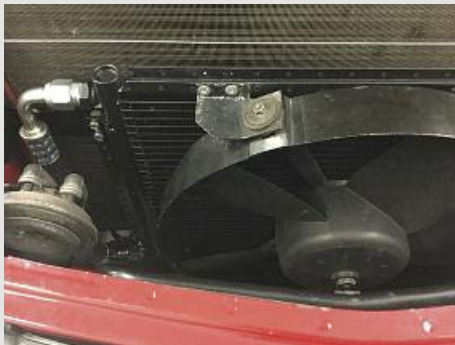
Condenser in front of the radiator
