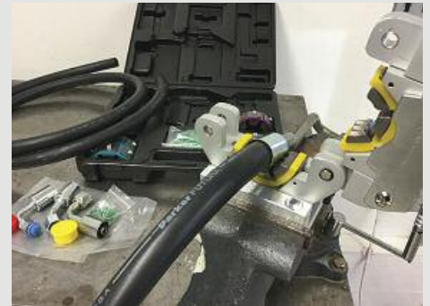
Crimping a fluid transfer hose
