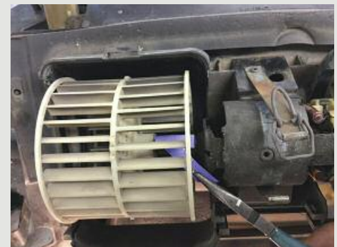
Where there should be foam insulation
