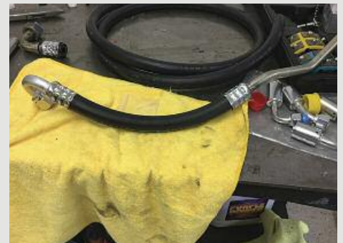
Hose with fittings after being crimped
