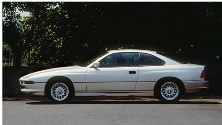
That's the middle pillar at the end of the front side windows, and BMW designed the 8-Series without it, allowing a clean sweep of glass from front to back. Cleaner, cooler.
