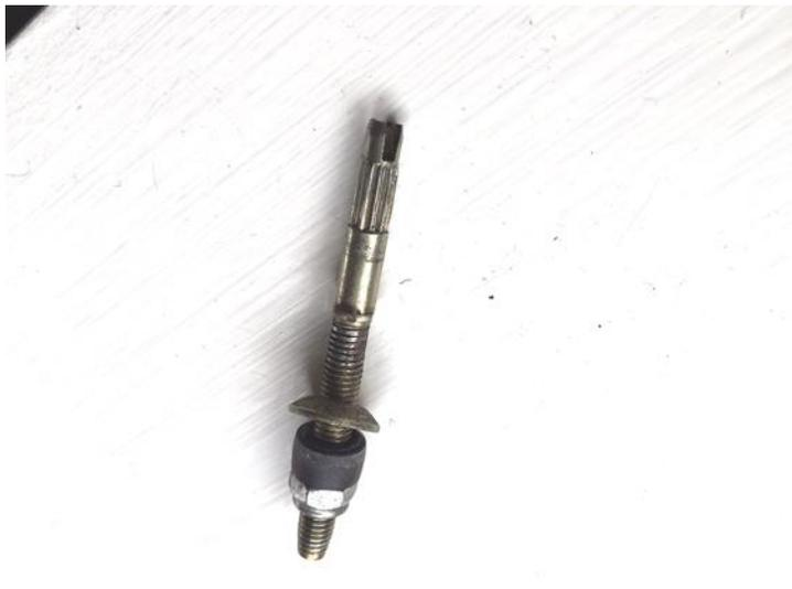
Next screw the 5mm nut onto the adjusting screw almost all the way, then put a washer under the nut and place on a vice with the jaws spread 1/4 inch. Next using a 13mm socket and a hammer tap the gear onto the adjusting screw until the slot end is level with the top of the gear. Don't have a vice? Drill a deep 1/4 inch hole into a 2X4 and tap away! Then using the screwdriver spread the slot like before. With the slot spread the gear can never slide off.
