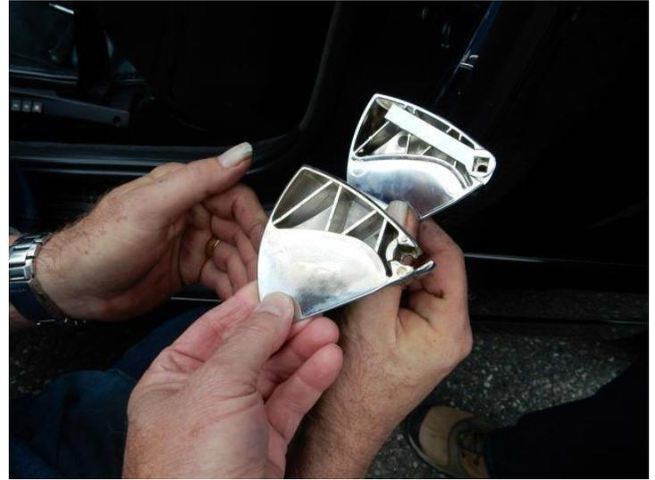
*E31 seat flipper - redesigned (on top) vs broken unit*
