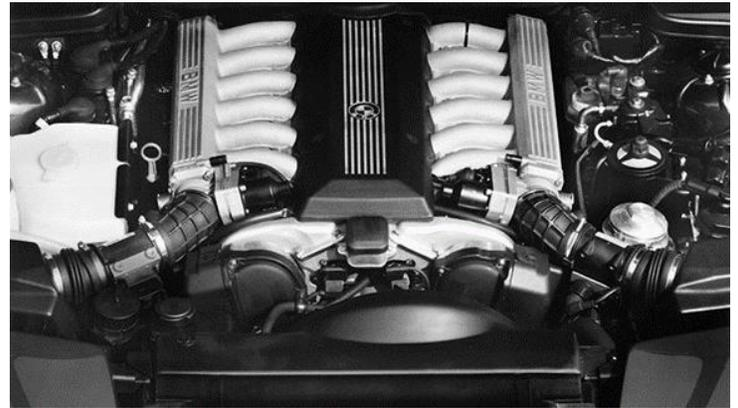
In 1993, BMW realized that 300 horses in something weighing 1790kg wasn't going to cut it with the Wolf of Wall Street crowd. So they ramped up the capacity of that V12 from 5.0 liters to 5.6 liters, tweaked to produce 381bhp and 406lb ft. Meet the 850 CSI, which was only available with a manual gearbox. That new-found power was enough to cut the 0-62mph sprint down from 6.8 seconds to under six seconds. Much more like it.
