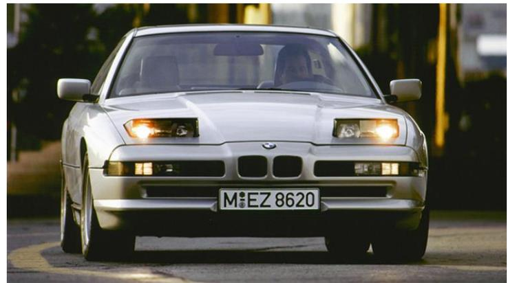
In 1994, BMW shuffled its 8-Series cards; with the range-topping 850 CSI coming on tap, the old 850 was dropped, its place filled with a new 850 CI with a 5.4-litre V12, 326bhp and a new five-speed auto.
