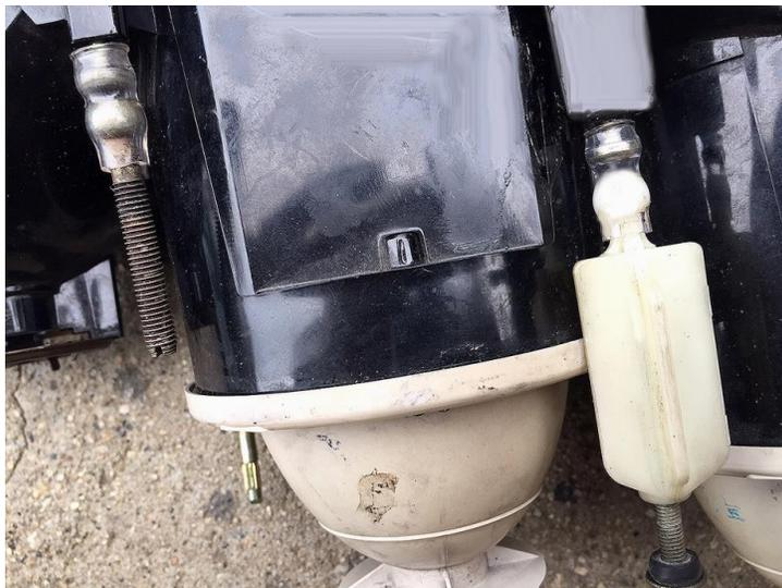
What you have done is to replace the hard plastic parts that are known to brake and fail with plastic tubing that is flexible and very long lasting. It takes a lot of force to pull the tubing off so it is not likely they will ever fail. The tubing also insulates the headlight from vibration and is a simple proven solution used by BOSCH and HELLA for many years and a simple and very inexpensive cure to an extremely common and expensive E31 headlight problem.
