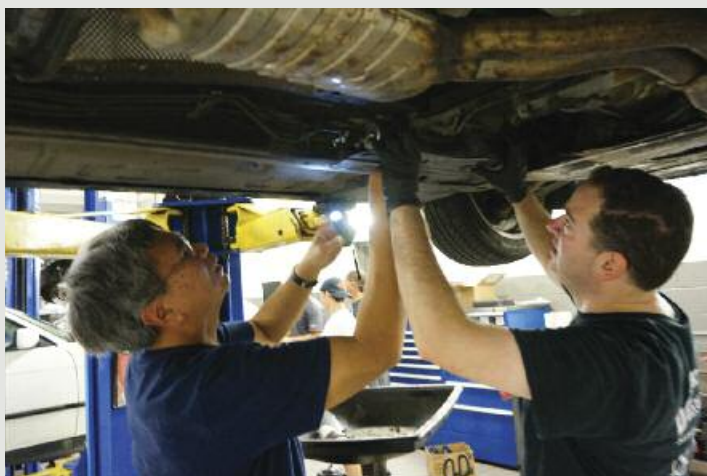
(Top) Chris Wootten shows DIY Coordinator Phillip Cummings how to remove the side valence on an E28 and replace the gasket underneath. Phillip will be doing this on his E28 M5 at a future event. (Above) Ed Darden replaced the front brake pads and rotors on his 2006 750Li.
