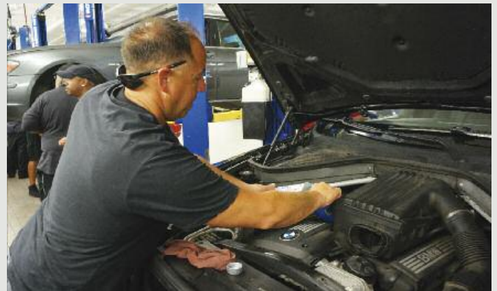
(Top right) In preparing to flush the brake fluid on his E46 ZHP, Mario Rodriguez carefully laid out some towels to protect his car. Brake fluid can eat the paint right off your car if not cleaned up after a spill. (Above right) Patrick Dietz changed the oil on his 2008 X5.
