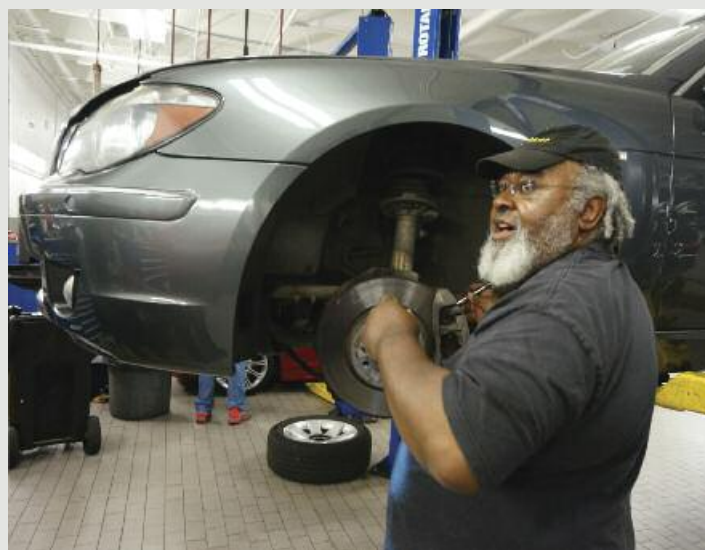
(Top) Chris Wootten shows DIY Coordinator Phillip Cummings how to remove the side valence on an E28 and replace the gasket underneath. Phillip will be doing this on his E28 M5 at a future event. (Above) Ed Darden replaced the front brake pads and rotors on his 2006 750Li.
