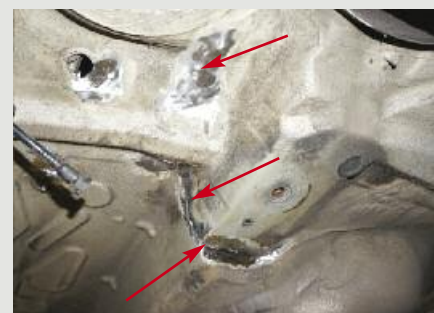
(Top) Mark Shaffer replacing the front brake pads and rotors on his 5 Series. (Middle:) Frank Kapitan tightens the lug nuts on his X3. (Bottom) At Speed had to grind the areas of this E46 M3 exhibiting subframe cracks (see the arrows) in preparation for welding in a reinforcement kit.
