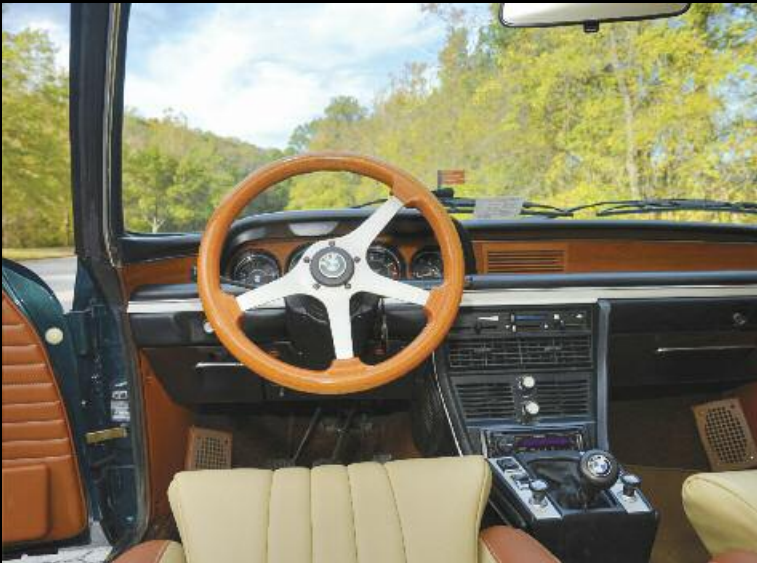
(Top) The huge glass area, combined with pillar-less window design, makes it almost convertible-like. A smallish sunroof was an option, but it led to roof rust problems. (Left) Installations of an original Behr A/C unit with rotary compressor and a sportier steering wheel add comfort and driveability. (Below, from left) The original engine, overbored and rebuilt, resides in an upgraded engine compartment. Scheel-Mann front seats are supremely comfortable and are mechanically adjustable for lumbar support – a real plus on a long trip. The interior color combo is original.
