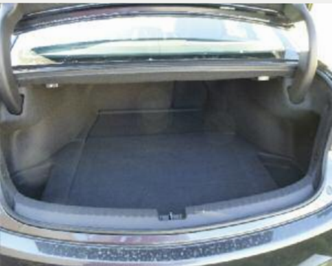
(Top and above) There's a German vibe with the Acura TLX interior. Honda's clever engineering is evident with the TLX's stowaway trunk lid supports.
