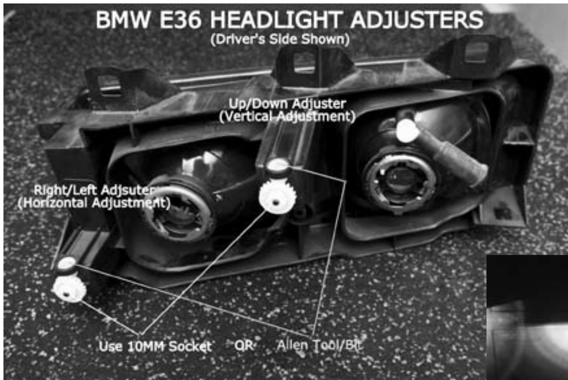
Fig. 1 - Backside of the E36 headlight assembly (driver's side) highlighting the adjusters for dialing in the aim of the headlight beams. Inset Image (R) - Headlight pattern reflected off a vertical surface showing the distinctive "vertical cut-off angle" described above.
