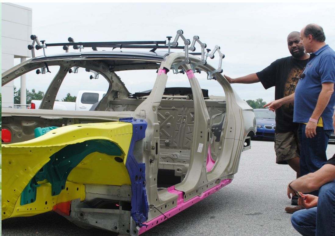
Dwayne Mosley and Tim Dennison (l,r) learning about this rolling shell F01 7-series. It is used for STEP training and the third man pictured developed the idea of color-coded sections to better train BMW mechanics for body repairs. Great idea!
