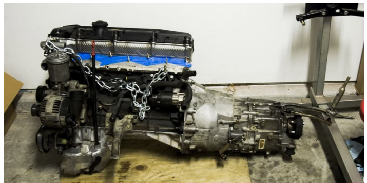
New Motor and Transmission Ready for Installation
