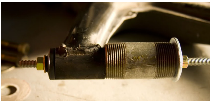
Alternate Special Tool for Removing Bushings
