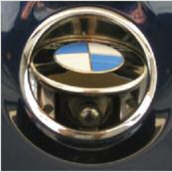
(Above) The trunk-mounted roundel tilts to reveal the nicely hidden backup camera - though a laser, rocket launcher, or oil canon would have been a lot cooler.
