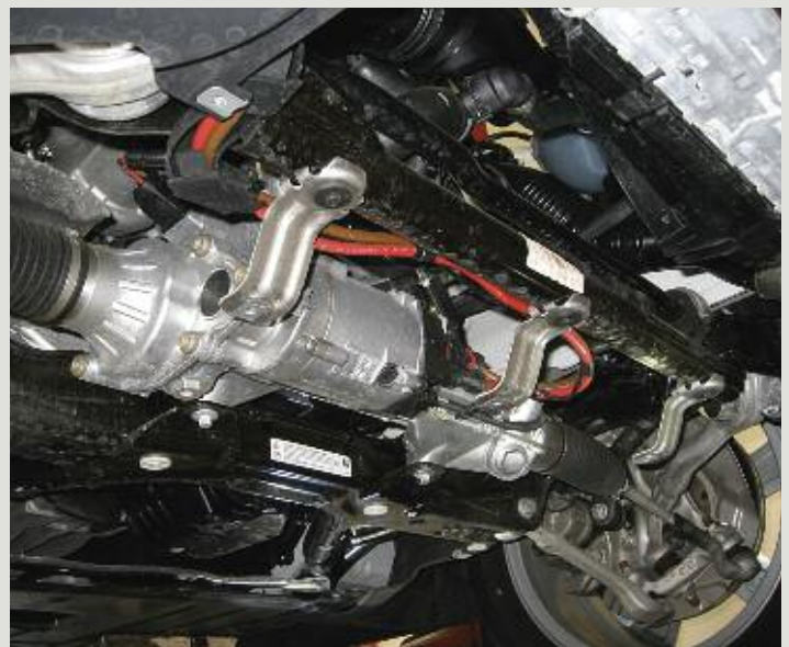
(Right top) The large plastic engine cover hides the new twin turbo four-cylinder engine. (Below) The new electronic power steering was designed to accommodate the new auto engine stop/start EfficientDynamics operation.
