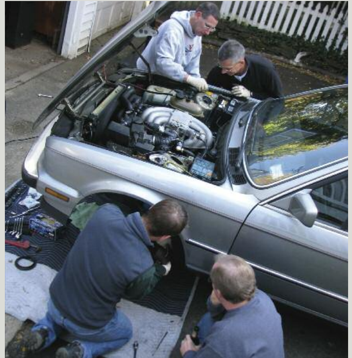
(Above Left) Marshall Lytle and Jim Gerock were able to compress the spring and remove the strut without having to remove the entire strut assembly from the car. (Above Right) Marshall and Jim (top) worked on removing one strut and spring on Marc Caden's 1987 325ic while Marc and John McWilliams (bottom) prepared the other side.
