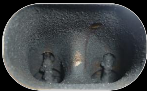
Before and after pictures of carbon deposit (“gunk”) in direct injection ports.
