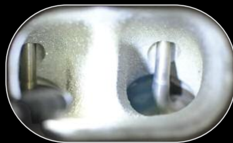
Before and after pictures of carbon deposit (“gunk”) in direct injection ports.
