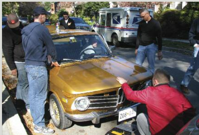
(Top) Dan Shor removed the front grills to reach in and unlatch the hood on Lou's 2002. (Left) After the latch was released, Dan and Marshall Lytle realigned the hood and ensured it was working properly.
