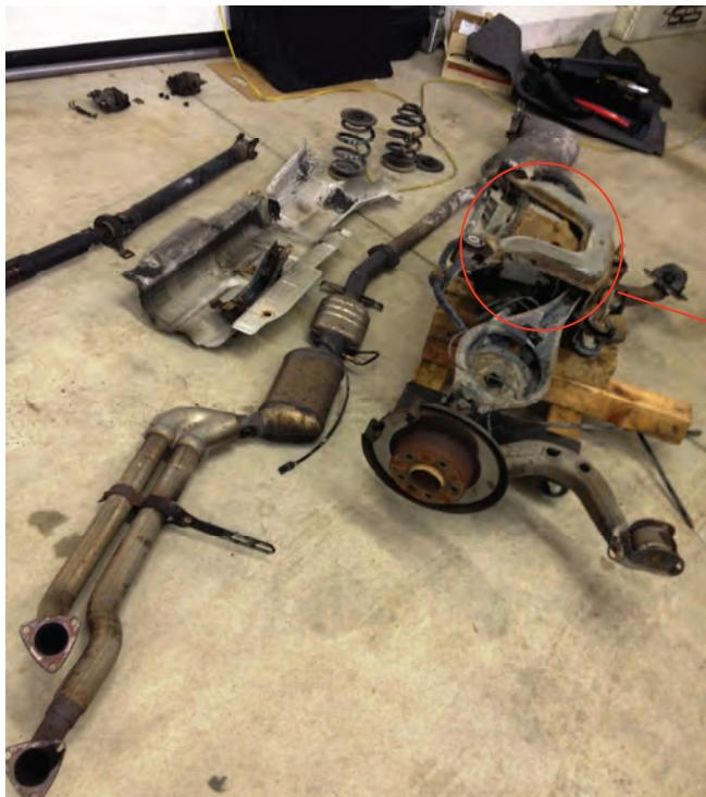
When the assembly is out of the car, we can remove the differential and then take off the upper wishbones (where the springs sit) and the lower control arms. Once the arms are removed we can press out the old bushings and press in the new ones. The outer bushings for these arms are located in the rear hub assembly; we use special BMW OEM tools to remove and then install these bushings. Here's a close-up of one of those well worn, 182,000 mile outer bushings.
