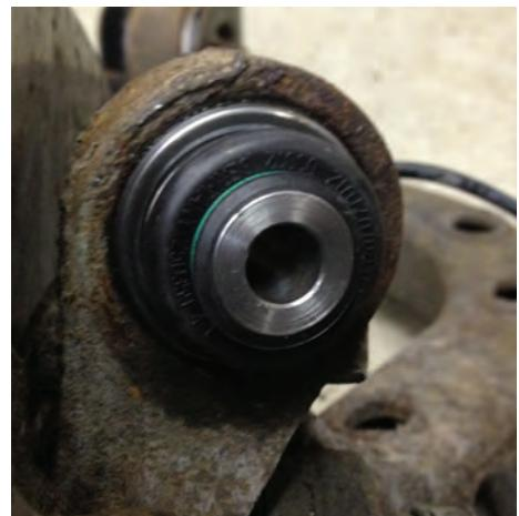
Once all the new bushings where pressed back into the suspension arms and sub-frame we re-assembled the rear end.
