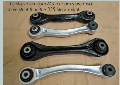
Top: M3 thrust arm Bottom: 335i thrust arm
