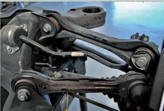
The rear subframe is out of the car, ready for rebuild.
