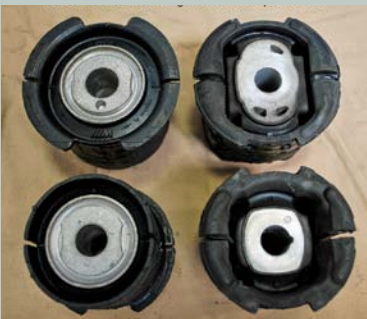
M3 subframe bushings on the left, compared to the 335i bushings. The solid M3 bushings help remove flex.
