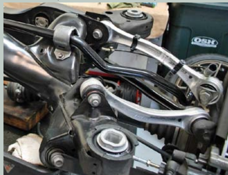
The rear subframe is rebuilt and ready to reinstall.
