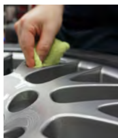
A good cleaning with a non-acidic wheel cleaner and dedicated wheel waxing will protect those wheels from brake dust and the harshest winters
